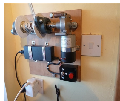
Hoisting a pulley full of clothes is impossible for clients with weak grips or arms. This modified windscreen wiper unit solves the problem.
